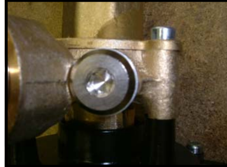
Figure 15b. Priming Screw Advanced
