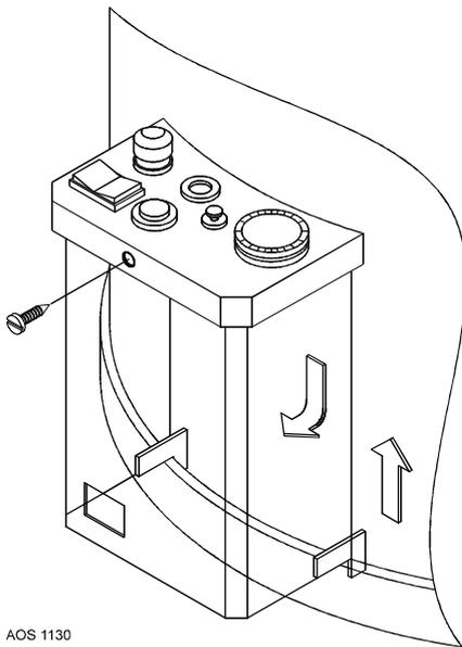
Figure 7 - Removing and replacing the control panel front cover
