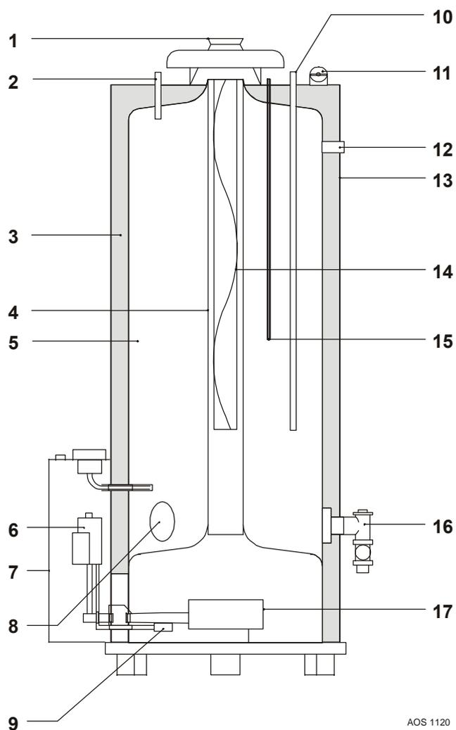
Figure 1 - Cross-section of the heater
