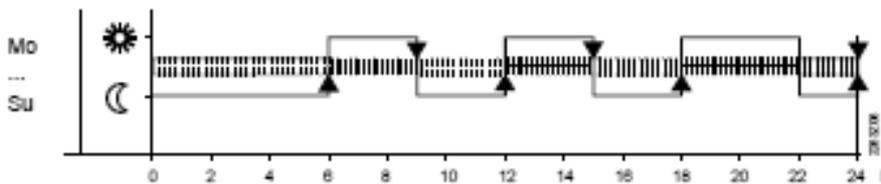
Comfort temperature and reduced temperature phases for heating circuit.
