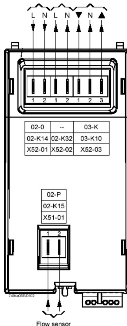
Connect the flow sensor, QAL36, supplied with the kit, using a twisted pair shielded cable, to terminals X51-01 on the second heating circuit clip-in relay.
