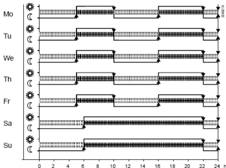
Tip: First, choose the 7-day block to enter the switching times required for the majority of days; then, select the individual days to make the required adjustments.
