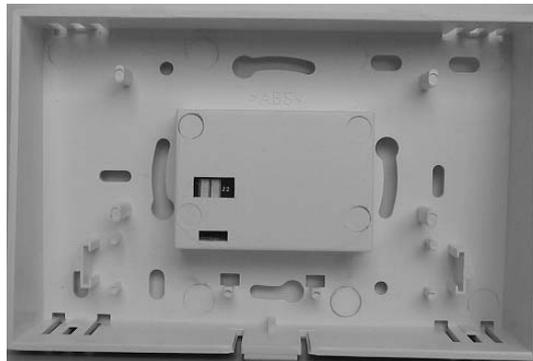
Engage the housing front at the top of the base and close the unit to the bottom.
