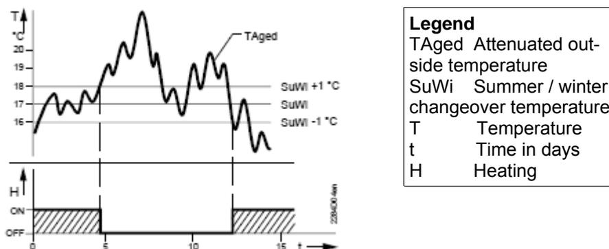
The 24-hour heating limit is used to switch the heating on and off in the course of the day, depending on the outside temperature. This function is used primarily during spring and autumn to respond to short-term temperature variations.
